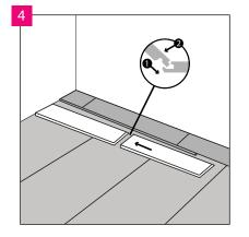
The floor panels are provided with locks on the short and long side. First, join the short sides of the neighbouring panels together.
