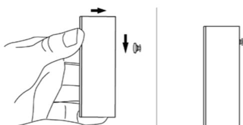
The CO sensor is activated automatically when it is installed on a wall or ceiling. When used as a free-standing device, it must be activated manually by pressing the installation screw supplied upwards in the installation hole.
